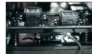
Lifting Capping Station
